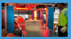
We can supply and integrate a wide range of static and dynamic DWS equipment, from camera to laser, 1-sided to 6-sided tunnels that are capable of scanning 1D and 2D bar codes.
