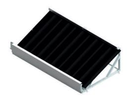
Constructed on a modular track, the articulating flites are mounted on connected carriages forming a continuous rotating sloped surface. The carriages are driven by a reliable caterpillar drive system. The modular design and construction allows for ease of installation and reconfiguration.
